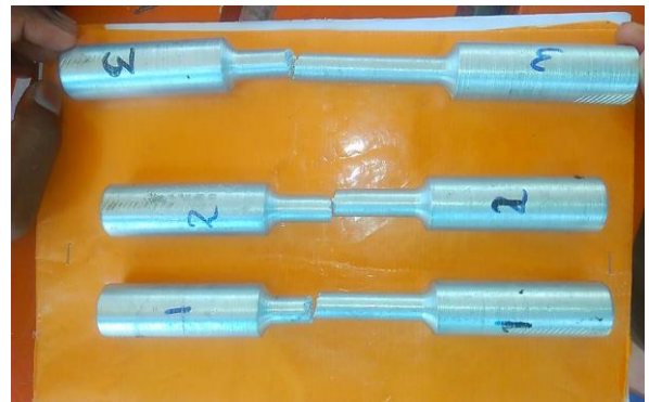
Figure 3. The specimen under the tensile test
