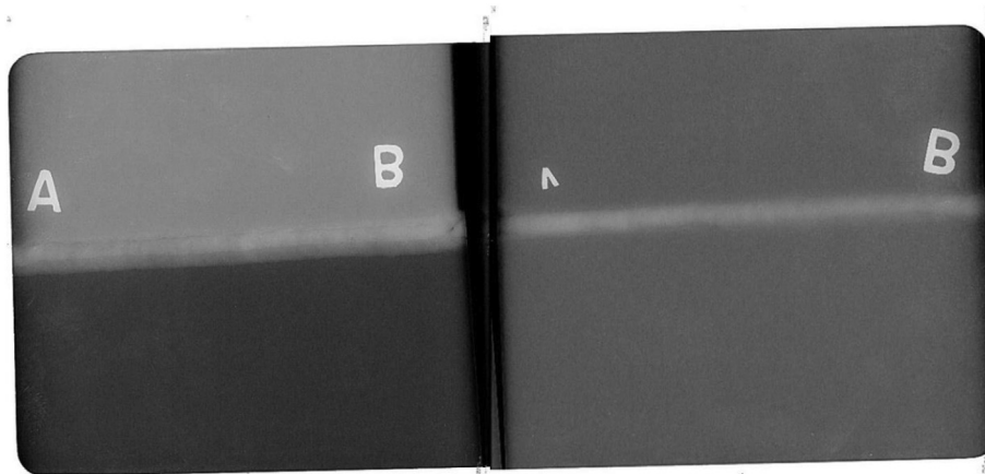
Fig. 2 – X-ray radiography images of dissimilar joint (left) CC-TIG and (right) PC-TIG welding processes.
